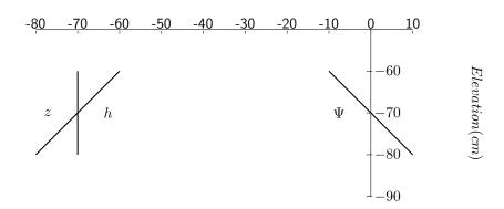
$$\begin{aligned} \mathbf{a} \quad & \Psi_{60} = z - \Psi_M - |\Delta z| = -60 + 90 - 20 = 10cm \\ & \Psi_{80} = -80 + 90 - 20 = -10cm \\ & |\Delta z|_{60} = 80cm \text{ and } |\Delta z|_{80} = 100cm \\ & h_{60} = z + \Psi + |\Delta z| = -60 - 90 + 80 = -70cm \\ & h_{80} = z + \Psi + |\Delta z| = -80 - 90 + 100 = -70cm \end{aligned}$$
