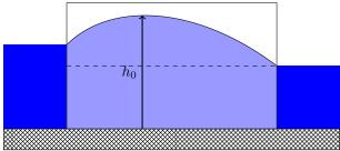
The recharge equation for unequal water levels applies here:  $h^2(x) = -\frac{N}{K}x^2 + C_1x + C_2$ Filling in the boundary conditions we get at x = 0  $h^2 = h_0^2 = C_2$ . Then at x = L we get  $C_1 = \frac{h_L^2 - h_0^2}{L} + \frac{NL}{K}$ .
