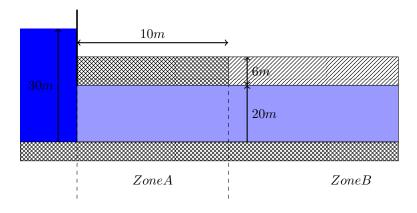
**a** In zone A  $h(x) = C_1 x + C_2$  applies. In zone B  $h(x) = h_a + C_1 e^{x/\lambda} + C_2 e^{-x/\lambda}$  applies.  $C_2 = 30m$  and  $C_1 = \frac{h_{10} - C_2}{10}$ . Therefore  $h_A = \frac{h_{10} - 30}{10} x + 30$
