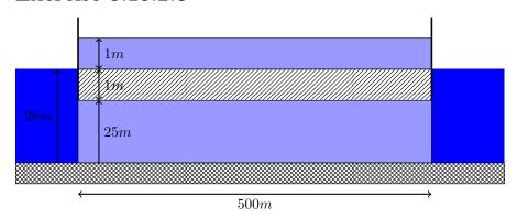
a The leaky flow equation,  $h(x) = h_a + C_1 e^{x/\lambda} + C_2 e^{-x/\lambda}$ , applies here. The vertical flow resistance c equals:  $c = \frac{d}{k} = 1/0,002 = 500$ . Therefore  $\lambda = \sqrt{Tc} = 500$ . Filling in the right boundary condition gives us  $C_2 = -1 - C_1$ . Then using the left boundary condition and substituting the value of  $C_2$  in the leaky flow equation we get  $C_1 = -0,2689$ . Therefore  $C_2 = -0,7311$ .
