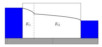
**a** For the left compartment:  $h^2(x) = C_1 x + C_2$ . Filling in the boundary conditions:  $x = 0 \rightarrow C_2 = 36$ .  $x = 40 \rightarrow C_1 = \frac{h_{40}^2 - 36}{40}$ .
