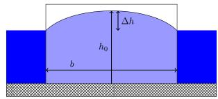
$T=KD=50m^2/day$  and  $\Delta h=0,09metres$  and N=0,01metres. By using the Hooghoudt equation we can solve for b, the distance between the two canals.  $N=\frac{\Delta h}{(\frac{L^2}{2KD_{average}})}$ .  $0,01=\frac{L^2}{(\frac{L^2}{2KD_{average}})}$
